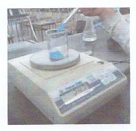
Add no more than half of the required volume of distilled water to the solute in the 100mL beaker. Stir with a stir rod until the solute is completely dissolved.
