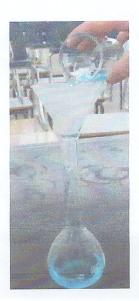
6. Add distilled water until the bottom of the meniscus reaches the etched line on the volumetric flask.
