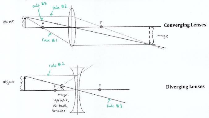
EXAMPLE: Determine the characteristics of the image using a ray diagram.
