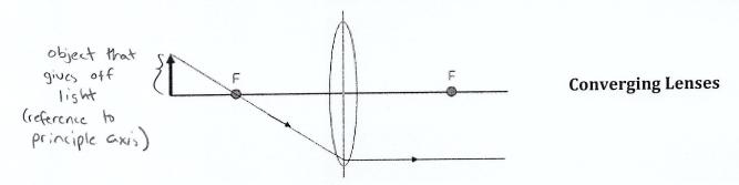
• Rule #2: Any ray parallel to the principle axis will refract so that is passes through the focal point. For a concave lenses, a ray will hit the lens and diverge/scatter. This means you need to extend the diverging ray to the focal point on the *opposite* side to the lens.
