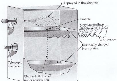
• When a voltage was supplied to the plates, some of the oil particles would rise to the top, some would remain suspended, and some particles would fall faster or slower to the bottom. All of these situations can be explained by the gravitational and electrical forces acting on the oil drop.
