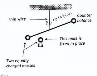
• The variables in Coulomb's torsion balance apparatus can be identified as:
