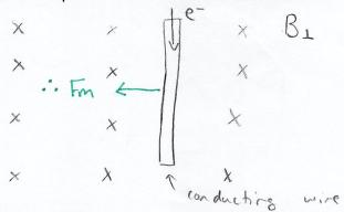
• The opposite is true as well. A <u>conductor forced to move through a magnetic</u> <u>field, can induce/produce an electrical current through the conductor</u>
