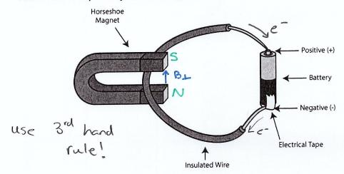
2. A 0.120 m long copper wire has a mass of 9.02g and is carrying a current of 5.10A perpendicular to a uniform magnetic field. This apparatus is placed in a strong magnetic field and the wire is found to levitate. Calculate the magnitude of the magnetic field strength.
